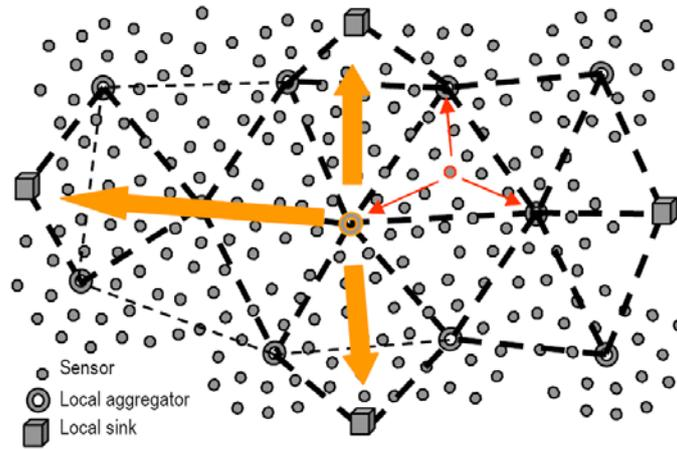
Figure 9. Underwater network topology [Seah and Tan, 2006]
