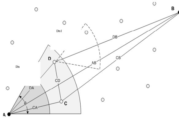
Figure.5. Illustration of the FBR protocol: nodes within the transmitter's cone  $\theta$  are candidate relays [Jornet, Stojanovic, and Zorzi, 2008]
