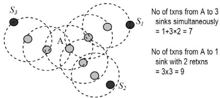
Figure 10. Multi-path Multi-sink/Virtual Sink [Seah and Tan, 2006]
