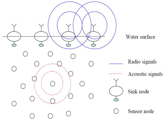
Figure 2. Multiple-sink underwater sensor network architecture [Yan, Shi, and Cui, 2008]
