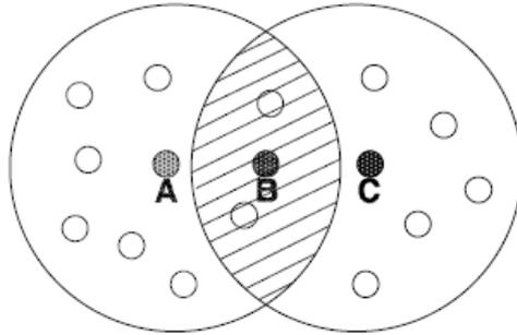
Figure 8a. A single forwarding community: any node in the shaded region can forward a packet between A and C [Lee et al., 2006]
