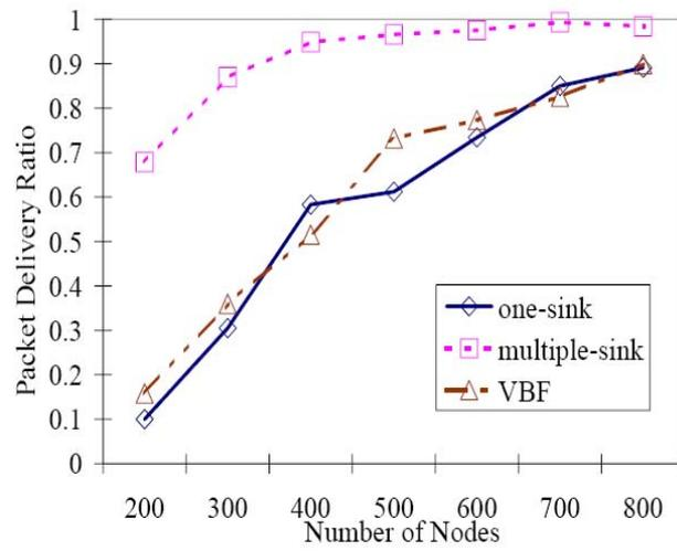
Figure 11(a). DBR vs. VBF according to packet delivery ratio [Xie, Cui, and Lao, 2006]
