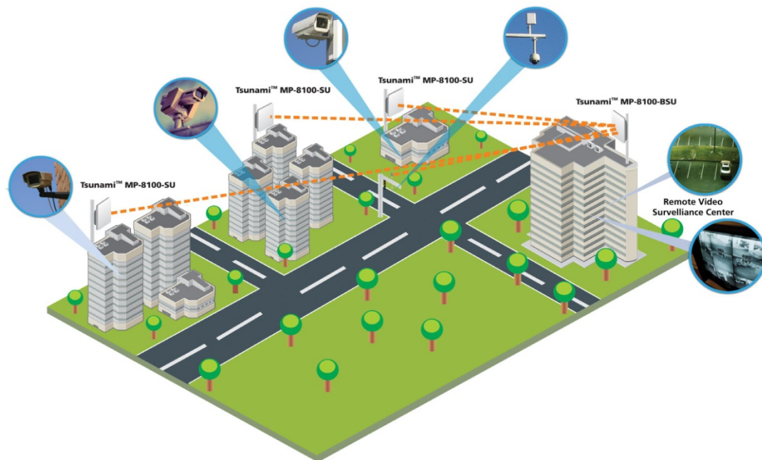
Σχήμα 1 Video Surveillance Backhaul using Tsunami™ MP-8100-BSU and MP-8100-SU
