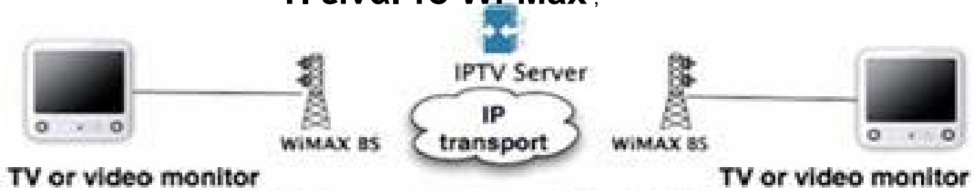
WiMAX as cable or satellite TV bypass
