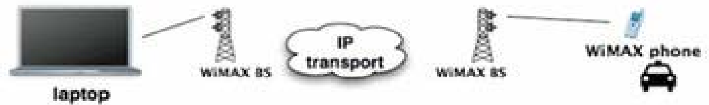
WiMAX as mobile data and cell phone bypass
