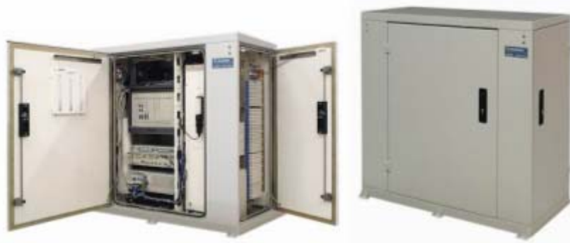
Figure : An outdoor IP DSLAM could be placed next to an ONU to provide EoVDSL
