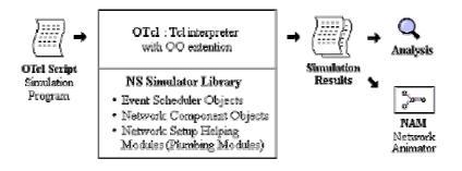
Tcl procedures are used to provide flexible and powerful control over the simulation (start and stop events, network failure, statistic gathering and network configuration). The Tcl interpreter has been extended (OTcl) with commands to create the networks topology of links and nodes and the agents associated with nodes.
