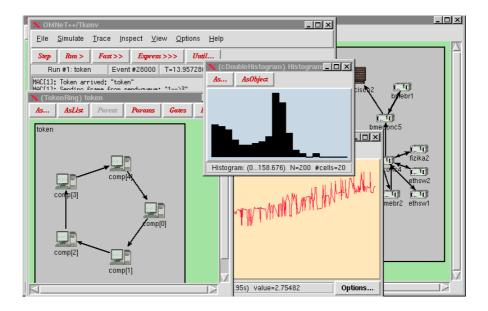
OMNeT++ simulations can feature different user interfaces for different purposes: debugging, demonstration and batch execution. Advanced user interfaces make the inside of the model visible to the user, allow him to start/stop simulation execution and to intervene by changing variables/objects inside the model. This is very important in the development/debugging phase of the simulation project. User interfaces also facilitate demonstration of how a model works.
