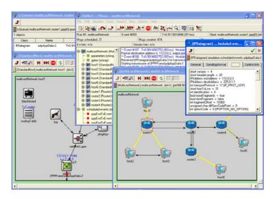
An OMNeT++ model consists of hierarchically nested modules. The depth of module nesting is not limited, which allows the user to reflect the logical structure of the actual system in the model structure. Modules communicate with message passing. Messages can contain arbitrarily complex data structures. Modules can send messages either directly to their destination or along a predefined path, through gates and connections.
